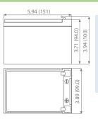
L: 5.95 in (151 mm) W: 3.89 in (99.0 mm) H: 3.71 in (94.0 mm) TH: 3.94 in (100 mm) Tolerances are +/- 0.04 in. (+/- 1mm) and +/- 0.08 in. (+/- 2mm) for height dimensions. All data subject to change without notice.
